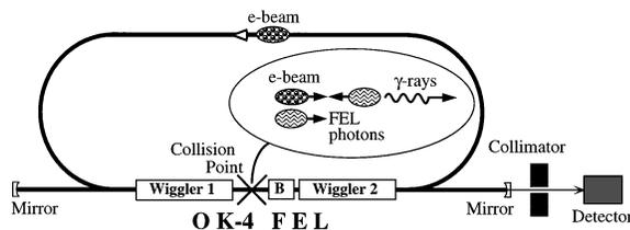
FIG. 1. Schematic of the OK-4/Duke storage ring FEL and  $\gamma$ -ray source. Two electron bunches spatially separated by one-half the circumference of the ring participate both in lasing and  $\gamma$ -ray production via Compton scattering of intracavity photons. A collimator installed downstream selects a narrow cone of quasimonochromatic  $\gamma$  rays.
