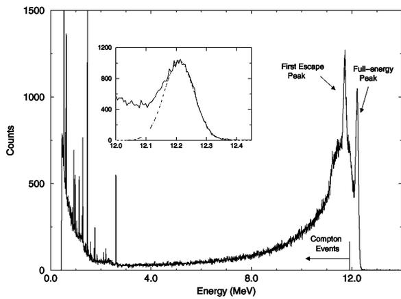
FIG. 2. Full  $\gamma$ -ray spectrum as measured by a HPGe detector. The full-energy and first escape peaks associated with the 12.2 MeV  $\gamma$ -ray beam are clearly visible. The inset shows a Gaussian fit to the full-energy peak. The fit has a FWHM of 120 keV.
