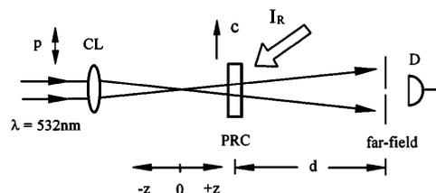
FIG. 1. Gaussian beam propagation configuration.
