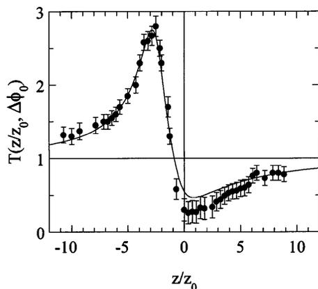
FIG. 2. Z-scan experimental results and the best theoretical fit (solid curve) with the parameters  $\Delta\phi_0 = 4.9$  and  $\beta_0 = 4.2$ .
