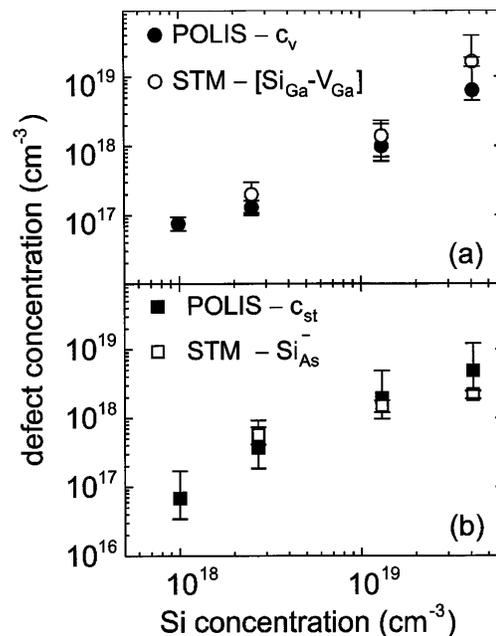
FIG. 3. (a) Concentrations of monovacancies from POLIS (filled circles) and  $\text{Si}_{\text{Ga}}\text{-V}_{\text{Ga}}$  complexes determined from STM images (open circles) as a function of the Si concentration. (b) The same for shallow positron traps (filled squares) and  $\text{Si}_{\text{As}}$  acceptors observed in STM images (open squares).
