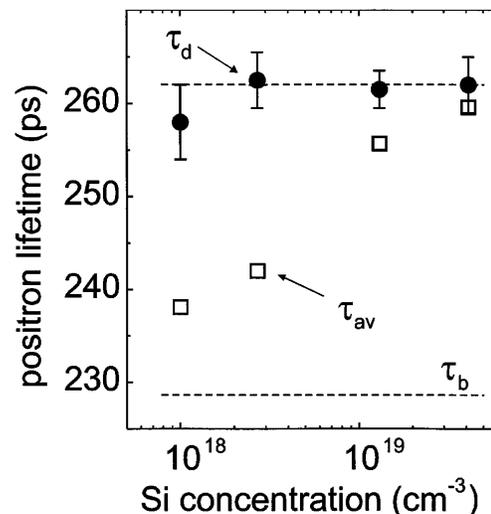
FIG. 1. Average positron lifetime  $\tau_{av}$  and defect related lifetime  $\tau_d$  as a function of the Si concentration (measured by SIMS) in Si-doped GaAs at room temperature.  $\tau_b$  is the positron lifetime in defect-free GaAs.
