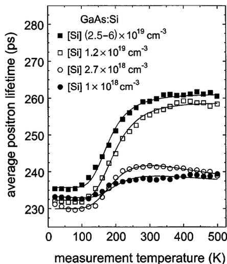
FIG. 2. Average positron lifetime  $\tau_{av}$  as a function of the temperature for different Si doping levels. Solid lines are fits to the experimental data with the assumption of positron trapping at negatively charged vacancies and negative ions.
