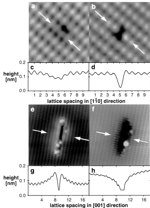
FIG. 4. Constant-current images of the occupied (a) and empty states (b) of a  $\text{Si}_{\text{Ga}}\text{-V}_{\text{Ga}}$  complex. (c) and (d): Line profiles along the atomic rows marked with the arrows in frames (a) and (b), respectively. (e) to (h): The same displays for a Si cluster.
