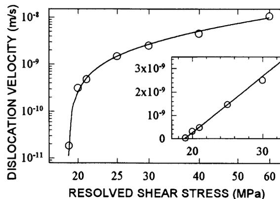
FIG. 2. The stress dependence of average  $60^\circ$  dislocations velocity. The inset shows the data replotted with linear axis to demonstrate the validity of the approximation used. Solid lines represent the results of fitting using Eqs. (1) and (3).
