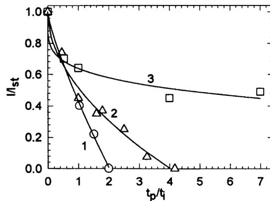
FIG. 3. The normalized dislocation displacement vs relative pulse separation:  $\sigma_p = -8$  MPa,  $t_i = 45$  ms (1);  $\sigma_p = -4$  MPa,  $t_i = 48$  ms (2);  $\sigma_p = 0$ ,  $t_i = 30$  ms (3). Solid lines are curve fits with Eq. (7).
