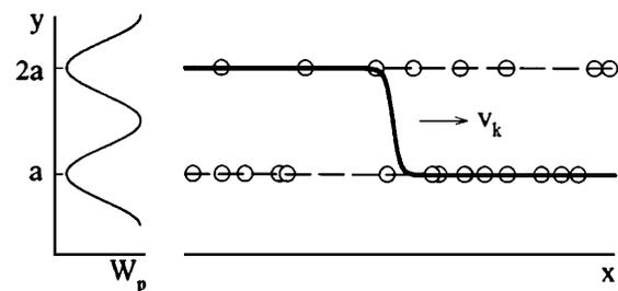
FIG. 1. The sketch of the dislocation kink.  $W_p(y)$  shows the Peierls relief, the circles represent randomly distributed point defects.
