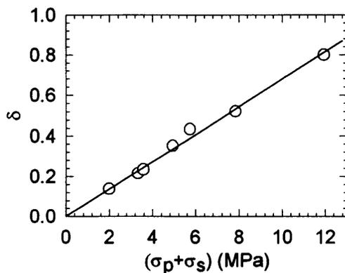
FIG. 4. Stress dependence of the parameter  $\delta$ .
