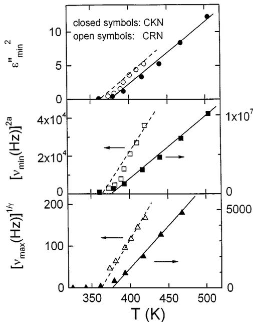
FIG. 4. Temperature dependence of height and position of the dielectric loss minimum and of the  $\alpha$ -peak position of KKN (closed symbols) and CRN (open symbols). Representations have been chosen that result in straight lines according to the predictions of the MCT. The solid lines are consistent with a critical temperature of  $T_c = 375$  K for KKN, the dashed lines with  $T_c = 365$  K for CRN.
