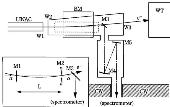
FIG. 1. Schematic layout of the experiment. BM: bending magnet; W1, W2: titanium windows; W3: aluminum windows; M3, M5: plane mirrors; M4: spherical mirror; WT: water tank (beam catcher); CW: concrete wall. The inset shows the open cavity composed of the mirror M1 of Al foil and the mirror M2 of a fused quartz whose central part of 20 mm in diameter is transparent. The trajectory of the electron beam is shown by the thin solid curve.
