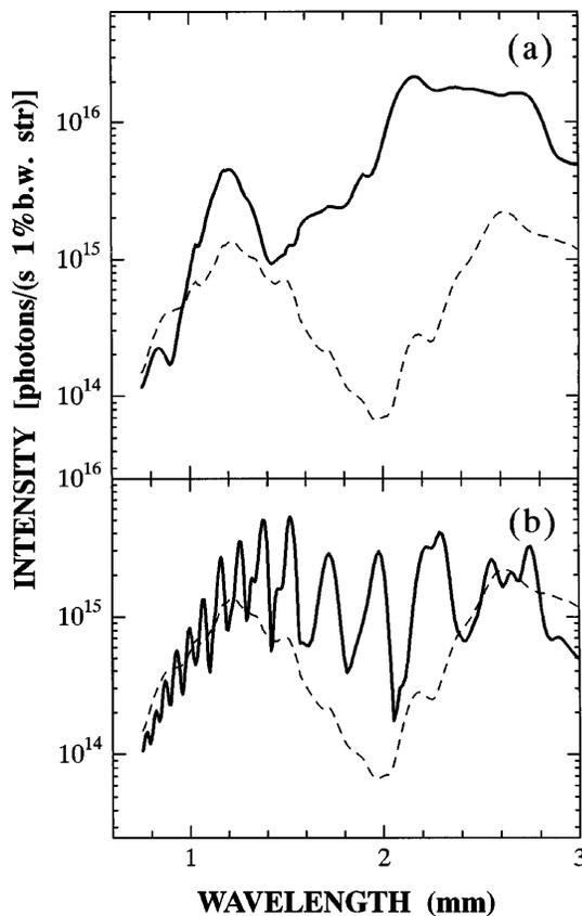
FIG. 3. (a) Spectrum observed at the whole resonance, i.e., the on-resonance condition (solid curve) for the whole harmonics. The dashed curve shows the spectrum at an off-resonance condition shown by the arrow  $a$  in Fig. 2. (b) Spectrum observed at a selectively resonant condition for particular harmonics with the cavity length shown by the arrow  $b$  in Fig. 2. The dashed curve shows the same off-resonance spectrum as in the upper figure (a).
