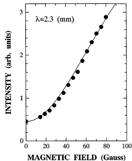
FIG. 4. Dependence of the intensity of the main peak on the magnetic field. Closed circles show the experimental result and the solid curve is the calculated intensity of a half-period undulator radiation in an arbitrary unit.
