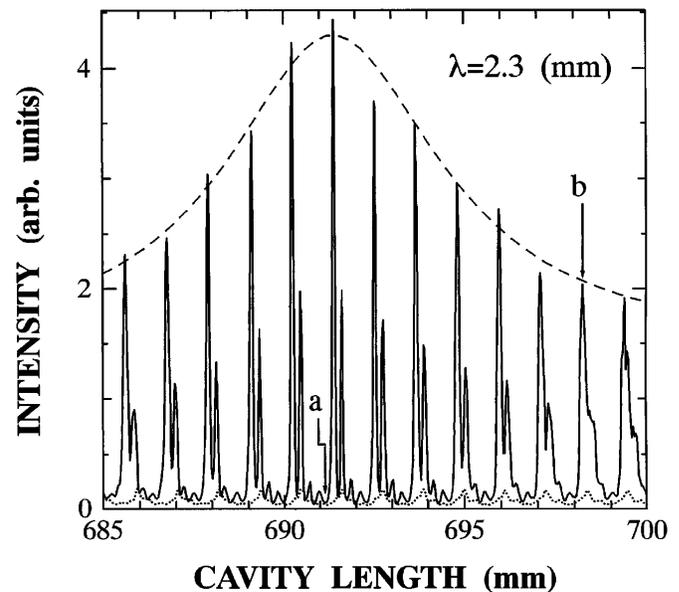
FIG. 2. Detuning curve of the intensity with the cavity length observed at  $\lambda = 2.30$  mm. The dotted curve shows the result obtained on the condition that the mirror M2 is tilted by  $2^\circ$  from the optimum direction. The dashed curve is the calculated envelope of the peaks with  $Q = 30$ .
