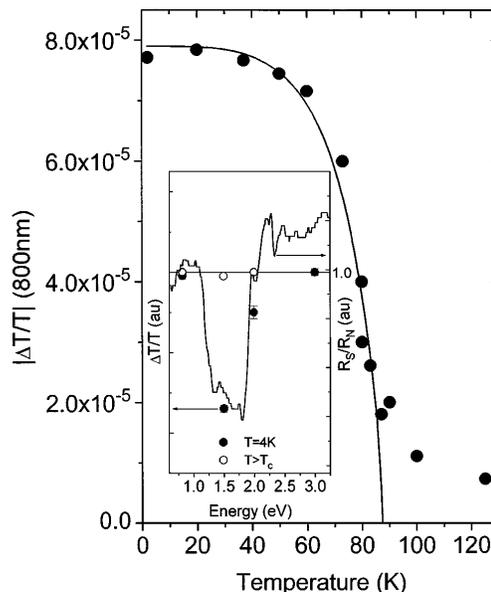
FIG. 4. Temperature dependence of the amplitude of the fast component in the differential transmittance. The solid curve is a fit to the two-fluid model for the gap function  $\Delta(\omega, T)$ . The inset shows a comparison of the TMS data with the dispersion of the amplitude of the fast signal, measured both above and below  $T_c$ .
