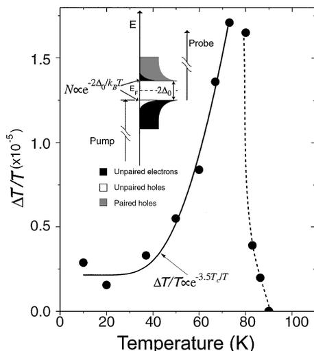
FIG. 5. Temperature dependence of the amplitude of the slow component in the differential transmittance. The solid curve is a fit to the data for thermally activated behavior. The broken curve is a guide to the eye, indicating the rapid decrease in the signal near  $T_c$ . The inset shows pump and probe optical transitions which can account for this behavior.
