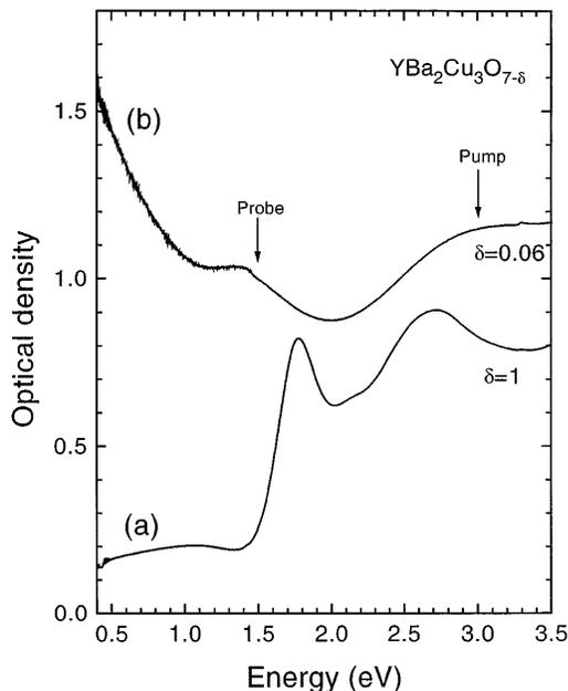
FIG. 1. Optical absorption spectrum of (a) insulating and (b) superconducting thin film  $\text{YBa}_2\text{Cu}_3\text{O}_{7-\delta}$  at 4 K. The arrows indicate the energies of pump and probe photons in the time-resolved measurements.
