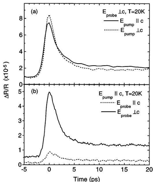
FIG. 3. Anisotropy of the differential reflectance of  $\text{YBa}_2\text{Cu}_3\text{O}_{7-\delta}$  crystals measured at 20 K.
