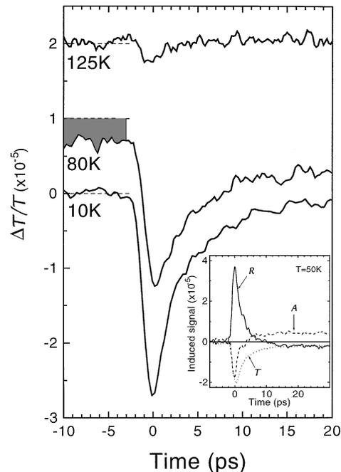
FIG. 2. Time-resolved differential transmittance of  $\text{YBa}_2\text{Cu}_3\text{O}_{7-\delta}$  thin film at temperatures above and below  $T_c$ . The traces are displaced for clarity of presentation, the broken line indicating the baseline. The inset shows curves for the differential reflectance (solid) and transmittance (dotted) and differential absorption (broken) obtained at 50 K.
