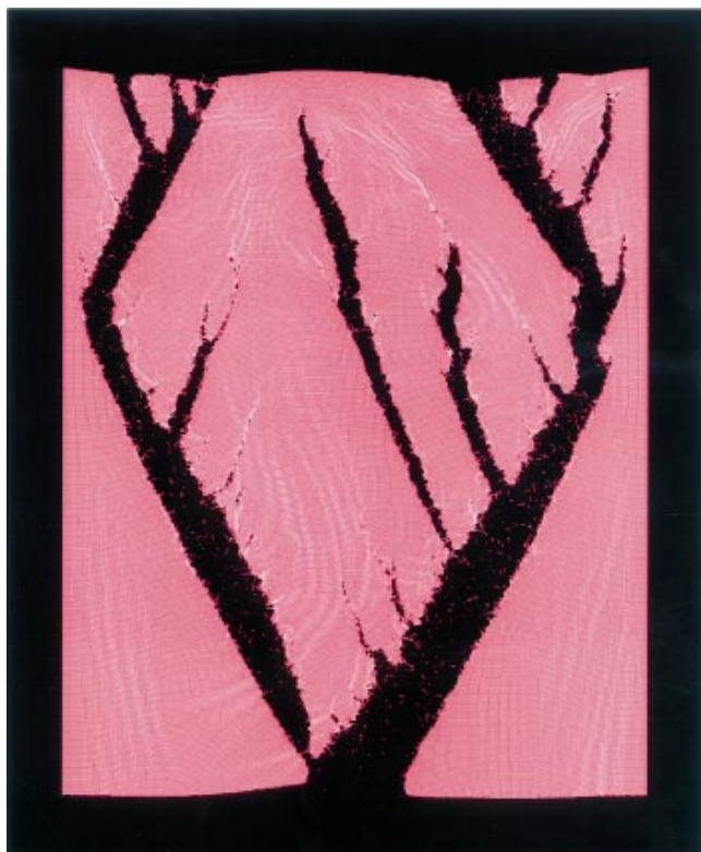
FIG. 3(color). Fracture in a graphite sheet subjected to 16% strain in the G(1,0) orientation.
