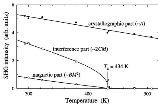
FIG. 3. Temperature variations of crystallographic, magnetization-induced, and interference terms in the SHG intensity for the (111) film.
