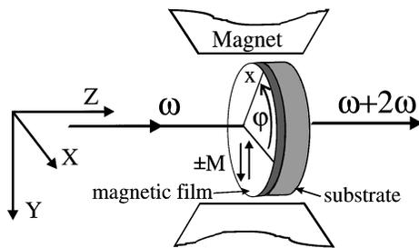
FIG. 1. Experimental geometry: sample rotates in a transverse magnetic field.
