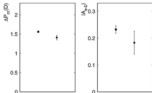
FIG. 4. Left panel: tensor polarization,  $\Delta P_{zz}(D)$ , of the atoms. Right panel: absolute value of the elastic electron-deuteron scattering asymmetry. Data are given for both the PTFE-coated aluminum (squares) and the uncoated copper cell (circles).
