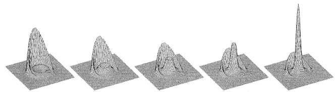
FIG. 4.  $Q(\alpha)$  for a weak drive ( $\Omega_R = 4\delta$ ,  $\omega = \omega_c - 50.2\delta$ ) decays at rate  $\gamma_{\text{loss}} \approx \gamma_c/4$  despite a large initial excitation to  $\bar{n} = 50$ , in sharp contrast to the stability expected classically.
