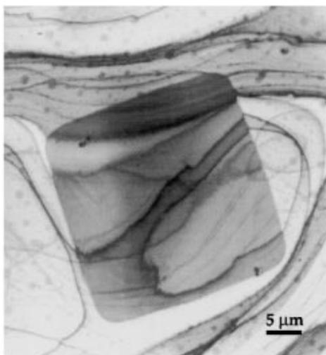
FIG. 1. Bright field TEM image of an epitaxial Fe(001) element supported on a GaAs single crystal membrane.
