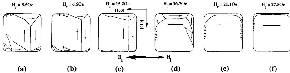
FIG. 4. Domain structures of the  $12 \times 12 \mu\text{m}^2$  epitaxial Fe element with edges parallel to the  $\langle 100 \rangle$  directions during reversal along the  $[100]$  easy axis.
