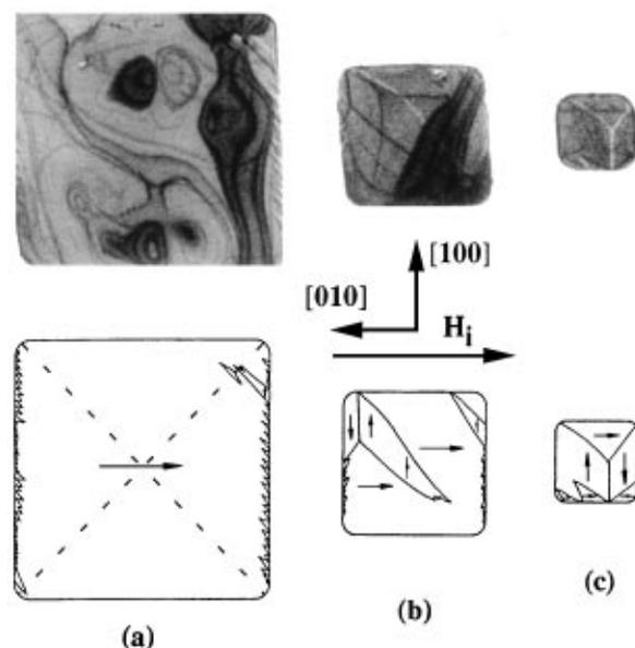
FIG. 2. Remanent domain images and corresponding magnetization schematics of the epitaxial Fe elements with edges parallel to the  $\langle 100 \rangle$  directions. The field was initially applied along the  $[0\bar{1}0]$  direction. The element sizes are (a)  $55 \times 55 \mu\text{m}^2$ , (b)  $30 \times 30 \mu\text{m}^2$ , and (c)  $12 \times 12 \mu\text{m}^2$ .
