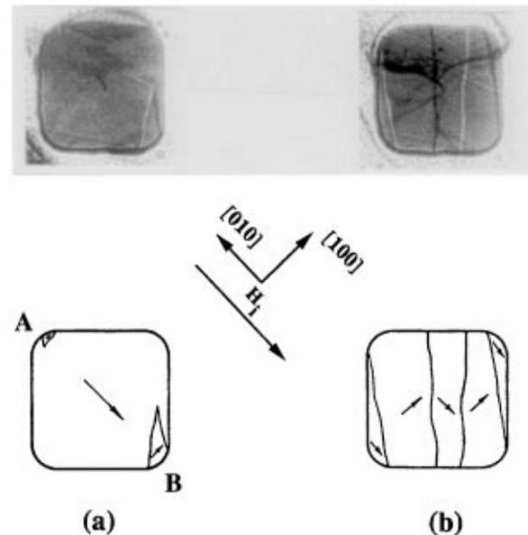
FIG. 3. Domain images and corresponding magnetization schematics of a  $12 \times 12 \mu\text{m}^2$  epitaxial Fe element with edges parallel to the  $\langle 110 \rangle$  directions. The field was initially applied along the  $[0\bar{1}0]$  easy direction. (a) Corner domain nucleation and growth upon reducing the applied field ( $H_i = 6.0$  Oe), (b) Remanent domain structure.
