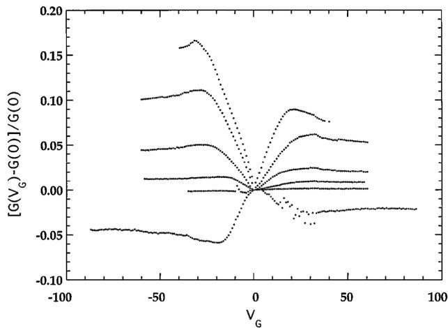
FIG. 2. Dependence of  $\Delta G/G(0)$  on  $V_G$  for a series of Pb films, with sheet resistances of 40, 25.34, 17.9, 11.31, 7.5, and 3.25 k $\Omega$ , where  $R_{\square}$  was measured at 24 K. The top curve shows the most resistive film, with  $R_{\square}$  decreasing for each subsequent curve.
