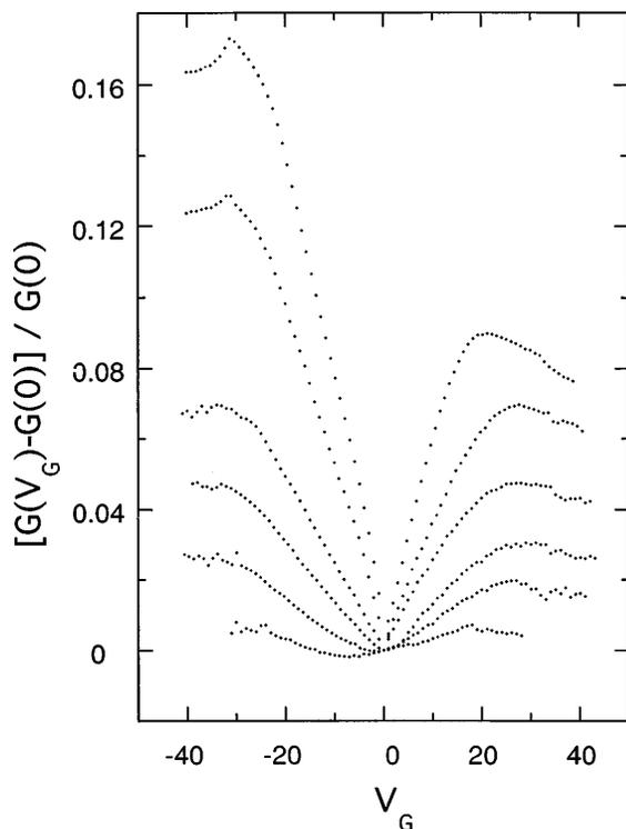
FIG. 1. Variation of  $\Delta G/G(0) = [G(V_G) - G(0)]/G(0)$  with gate voltage  $V_G$  and temperature  $T$  for a Pb film with a sheet resistance of 40 k $\Omega$  at 24 K. The temperatures from top to bottom are 2.3, 3, 5, 8, 12, and 24 K.
