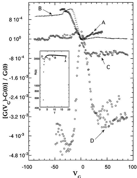
FIG. 3. Variation of  $\Delta G/G(0)$  with temperature for a Pb film with  $R_{\square} = 3.25$  k $\Omega$  at 24 K. The temperature decreases from top to bottom. Curves A through D correspond to data obtained at 18, 8, 4, and 3.0 K, respectively. Data obtained at other (lower) temperatures have been omitted for clarity. Shown in the inset is a plot of  $R_{\square}$  vs  $T$  on which the approximate position of curves A through D are indicated.
