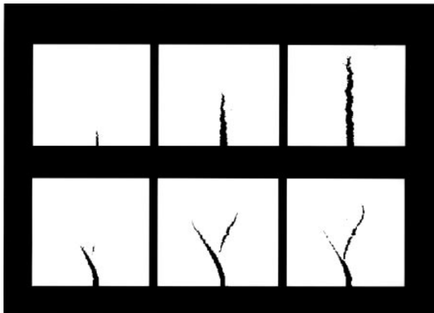
FIG. 2. Past simulations using the original LJ potential (see Ref. [4]); a black and white rendering is used to show the time evolution of the propagating crack through the solid slab. The time sequence goes from left to right. The top row is for the crack initially moving in the stiff direction, and the bottom row is for the crack initially moving in the soft direction. The system is \sim 5 \times 10^5 atoms.
