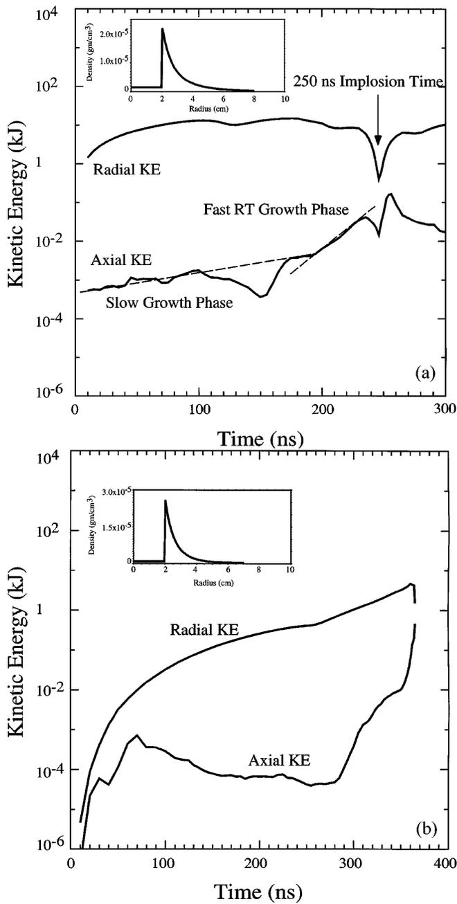
FIG. 1. Radial ( $KE_r$ ) and axial ( $KE_z$ ) kinetic energies vs time for implosion of a load with a constant current (a) and constant voltage (b). Initial density profiles are shown in the insets. Stagnation occurs at  $t = 250$  ns (a) and at  $t = 360$  ns (b).
