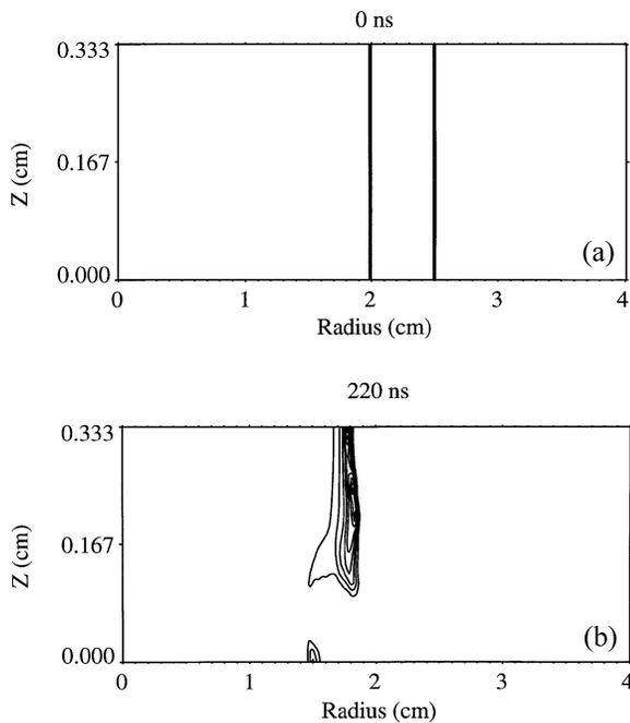
FIG. 3. Density contours for a shell which initially extends from 2 to 2.5 cm: before implosion (a) and at  $t = 220$  ns (b).
