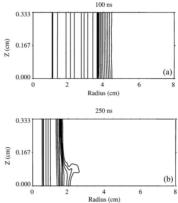
FIG. 2. Density contours corresponding to slow growth phase  $t = 100$  ns (a) and rapid growth phase  $t = 250$  ns (b) in Fig. 1(a).
