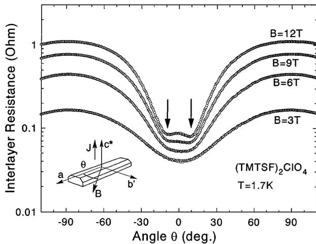
FIG. 3. Angular dependence of the interlayer MR in  $(\text{TMTSF})_2\text{ClO}_4$  when the magnetic field is rotated in the most conducting plane ( $\mathbf{a}\text{-}\mathbf{b}'$  plane). Arrows indicate the kink structures due to the third angular effect.
