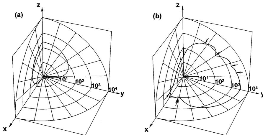
FIG. 1. Calculated angular dependence of the diagonal resistivity elements in the Q1D system.  $\pi/(\hbar^2/2t_a a^2 eB) = 20$  is assumed. (a) Normalized interchain resistivity in the conducting layer  $\rho_{yy}/(\pi abcB/2e)$ . (b) Normalized interlayer resistivity  $\rho_{zz}/(\pi abcB/2e)$ . Arrows in the  $y$ - $z$ ,  $x$ - $z$ , and  $x$ - $y$  plane indicate the Lebed resonance, the Danner-Chaikin oscillation, and the kink structure of the third angular effect, respectively.
