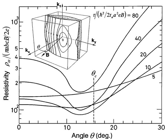
FIG. 2. Dependence of the third angular effect on the parameter  $\tau/(\hbar^2/2t_a a^2 eB)$ . The field angle is measured by the angle  $\theta$  between the 1D axis and the magnetic field direction. Dashed line indicates the critical angle  $\theta_c$  calculated by (5). Inset: Semiclassical electron orbits on the sheetlike FS's under the magnetic field.
