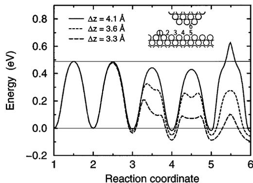
FIG. 3. Variation of potential energy when an adatom diffuses on a surface underneath a tip. The three curves correspond to three different tip-adatom separations,  $\Delta z$ . [ $\Delta z$  is the relaxed height difference when the adatom is in position 5 underneath the tip.] Inset: Side view of a part of the system.
