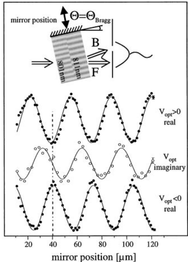
FIG. 4. Measurement of the sinusoidal distribution of the standing atomic wave field. The anomalously transmitted wave field (middle trace) has its maxima at the nodes of the standing light field. If the 801 nm standing wave is shifted off resonance, the standing atomic wave is shifted by  $\pi/2$  to the left for blue detuning (positive potential) and to the right for red detuning (negative potential).
