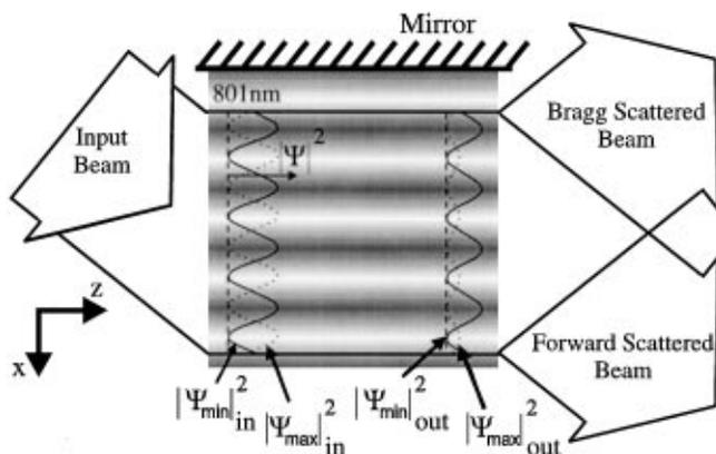
FIG. 2. Standing atomic wave fields for *exact* Bragg incidence inside the standing light field (lower standing light wave intensity represented by darker shading). Initially, the wave field inside the crystal is an equal superposition of  $\Psi_{\min}$  and  $\Psi_{\max}$  as indicated ( $\Psi_{\text{total}}^{\text{in}} = \Psi_{\min} + \Psi_{\max}$ ). Since the absorption is periodic  $\Psi_{\max}$  dies out faster than  $\Psi_{\min}$ .
