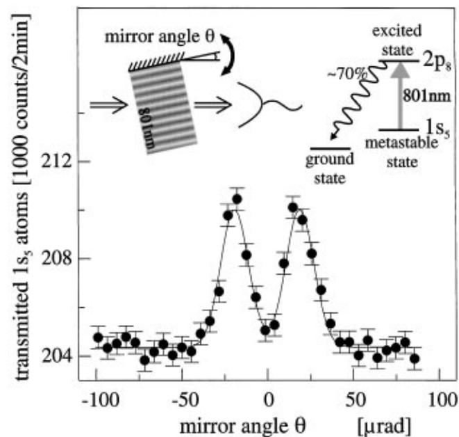
FIG. 1. Total intensity of the metastable  $\text{Ar}^*$  beam after transmission through a standing light wave tuned exactly on resonance to an open transition (see inset) as a function of incidence angle. The transmission increases anomalously for Bragg incidence from either side relative to the planes of the standing light field. The solid line is a fit curve with two Gaussian curves.
