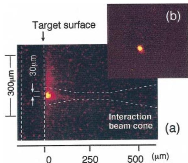
FIG. 4(color). X-ray pinhole camera images from (a) the target tangential and (b)  $10^\circ$  to the target normal. The dotted line shows a cone of the incident laser light at 250  $\mu\text{m}$  from the target surface.
