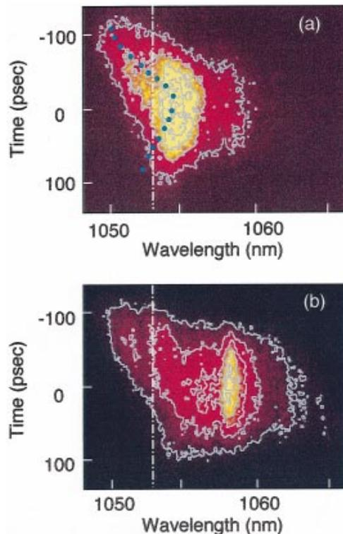
FIG. 1(color). Linear intensity contours of the time-resolved spectra of the backscattered light at the focus positions of (a) 100  $\mu\text{m}$  and (b) 250  $\mu\text{m}$ . The dotted lines correspond to the fundamental wavelength. The closed circles in (a) are estimations of Doppler shifts due to critical surface moving inward by the photon pressure.
