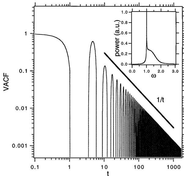
FIG. 1. Positive side of the velocity RF and corresponding power spectrum (inset) for the symmetric Duffing potential  $V(x) = \frac{1}{2}x^2 + \frac{1}{4}x^4$  at  $\beta = 1$ .
