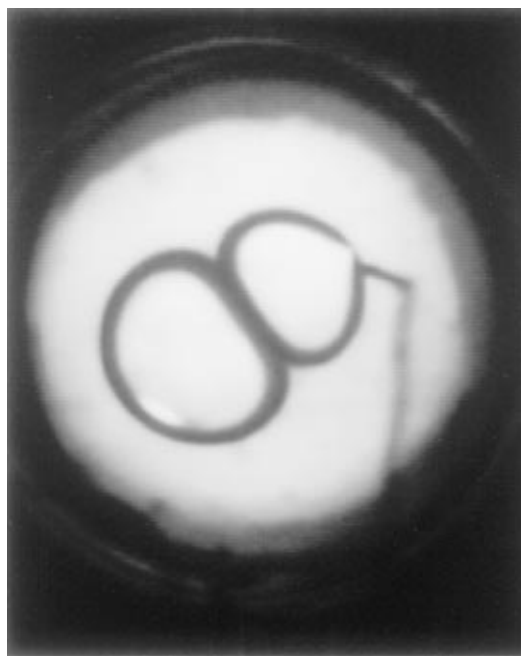
FIG. 2. Photograph of two drops in contact. The drops are viewed from above. The capillary which produced the two drops can be seen in contact with the drop on the right.
