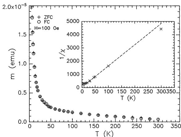
FIG. 3. Temperature dependence of induced magnetization at  $H = 100 \text{ Oe}$  for sample G2 field cooled and zero field cooled. Inset: inverse differential susceptibility  $1/\chi = dH/dM$  at  $H = 10 \text{ kOe}$  vs  $T$  for G3. Dashed line: fit to Curie law  $\chi = 0.06/T$ .
