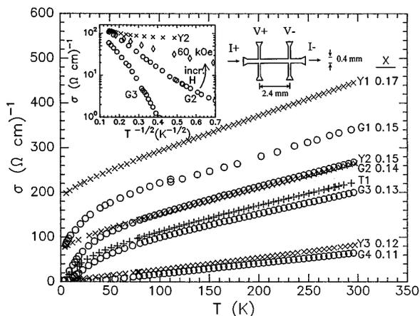
FIG. 1. Temperature dependence of conductivity for  $a\text{-Gd}_x\text{Si}_{1-x}$  (samples G1-G4:  $\circ$ ),  $a\text{-Y}_x\text{Si}_{1-x}$  (Y1-Y3:  $\times$ ), and  $a\text{-Tb}_x\text{Si}_{1-x}$  (T1:  $+$ ). Composition  $x$  is shown for each; uncertainty in  $x$  is  $\pm 0.01$ . Inset:  $\log_{10}(\sigma)$  vs  $T^{-1/2}$ .
