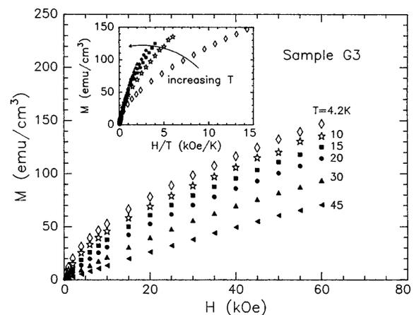
FIG. 4.  $M(H)$  for G3 for  $T < 50 \text{ K}$ .  $M_{\text{sat}} \approx 300 \text{ emu/cm}^3$ . Inset:  $M$  vs field normalized by temperature ( $H/T$ ).
