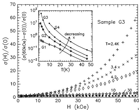
FIG. 2. Conductivity  $\sigma$  vs magnetic field for  $a\text{-Gd}_{13}\text{Si}_{87}$  (G3) at different temperatures [normalized to  $\sigma(0) =$  zero field value at each temperature]. Inset:  $\sigma$  at  $H = 60$  kOe  $-\sigma(0)$  normalized by  $\sigma(0)$  ( $=$  -magnetoresistance) versus temperature for G1-G4.
