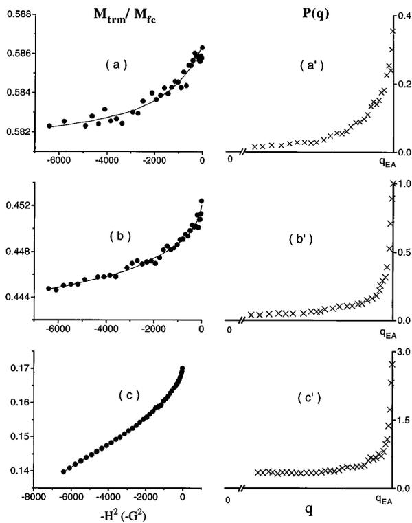
FIG. 3. Plots of  $M_{TRM}(t, t_w)/M_{FC}$  vs  $-H^2$  for Cu: Mn 6 at. % ( $T_g = 31.5$  K) at  $t = 10$  sec and  $t_w = 5$  min for (a)  $T_r = 0.13$ ; (b)  $T_r = 0.47$ ; and (c)  $T_r = 0.88$ . The solid lines are best fits to the data, the derivative of which with respect to  $-H^2$  is plotted to the right, giving  $P(q)$  from Eq. (5) in the text, with  $D = \frac{1}{2}(q_{EA} - q)$ .
