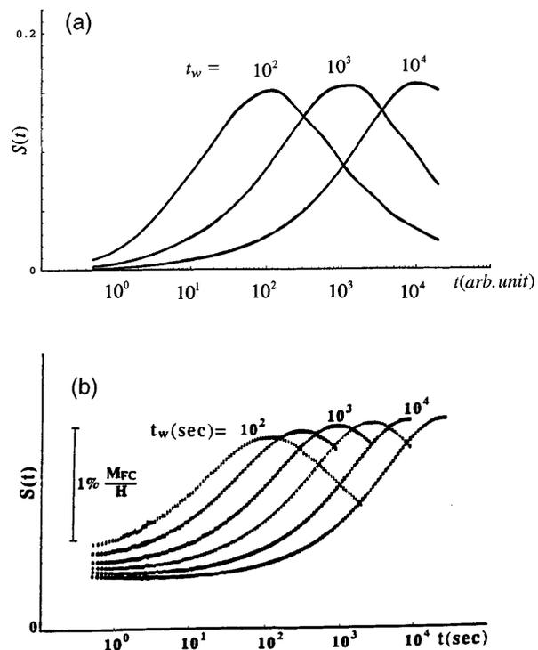
FIG. 1. (a) Using the finite bifurcating ultrametric tree for  $n = 20$ , we plot  $S(t)$  vs  $t$  for a three different waiting times. (b) Experimental values for  $S(t)$  from Ref. [10].
