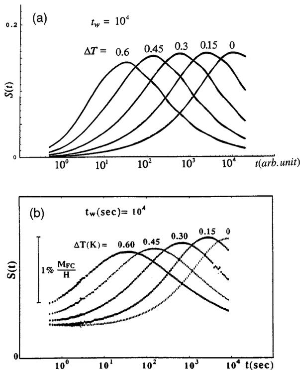
FIG. 2. (a) Plots of  $S(t)$  vs  $t$  for temperature cycling changes  $\Delta T(K) = 0, 0.15, 0.3, 0.45$ , and  $0.6$  according to the protocol of Ref. [13]. (b) Experimental values for  $S(t)$  for the same  $\Delta T(K)$  from Ref. [13].
