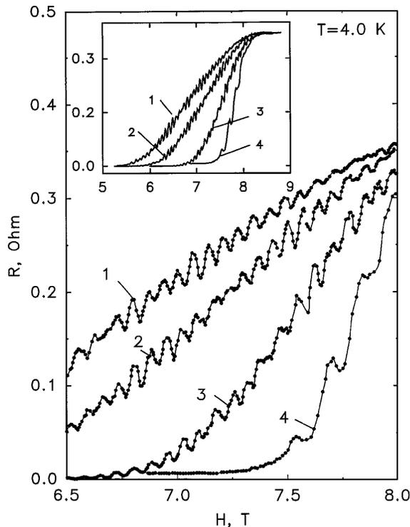
FIG. 1.  $R(H)$  curves for the NbTi/Cu multilayer with  $d_n = 10$  nm and  $d_s = 25$  nm for different  $j$  [A/cm<sup>2</sup>]:  $10^4$  (1);  $6 \times 10^3$  (2);  $2 \times 10^3$  (3);  $2 \times 10^2$  (4). Inset shows the same  $R(H)$  curves on a larger field scale.
