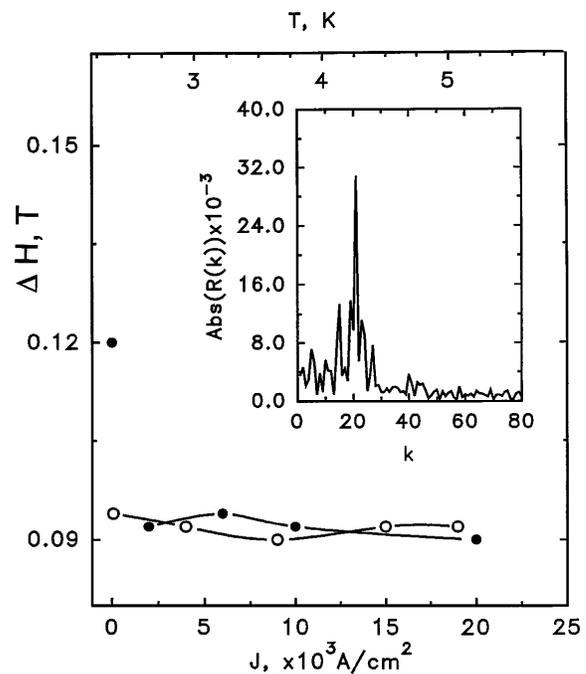
FIG. 2.  $\Delta H$  as a function of current density  $j$  (filled symbols) and temperature  $T$  (open symbols). Inset shows the Fourier transform of  $R(H)$  in Fig. 1, where  $k = 2.05/\Delta H$  [T]. The main peak in  $R(k)$  corresponds to  $\Delta H = 0.095$  T.
