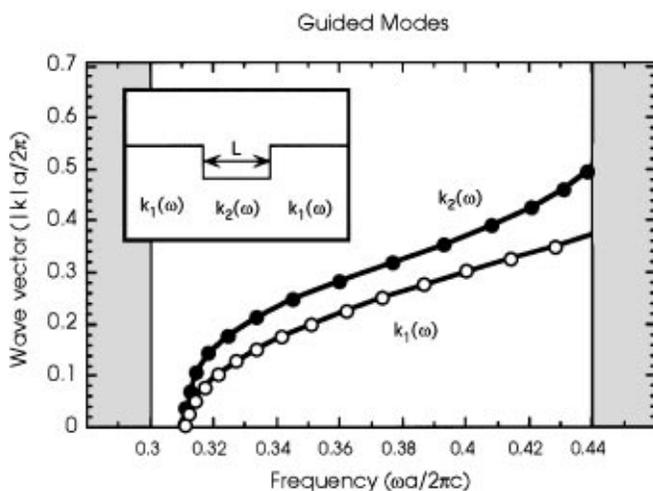
FIG. 3. Dispersion relation  $k_1(\omega)$  for propagation along the (01) or (10) direction, and  $k_2(\omega)$  for the (11) direction. The gray regions correspond to the edges of the band gap. The “potential” associated with the bend is shown in the inset.
