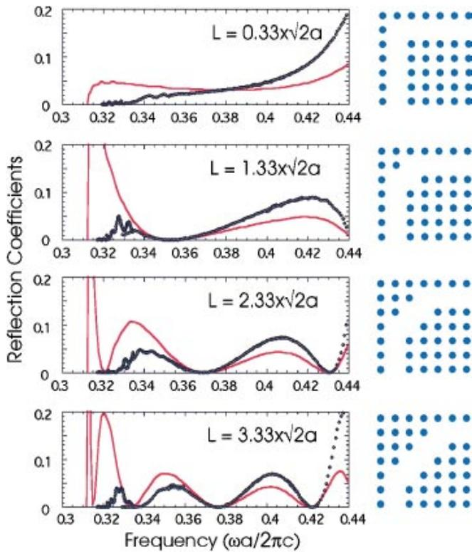
FIG. 4(color). Reflection coefficients computed from numerical simulations (diamonds) and from one-dimensional scattering theory (solid line), for four different bend geometries.
