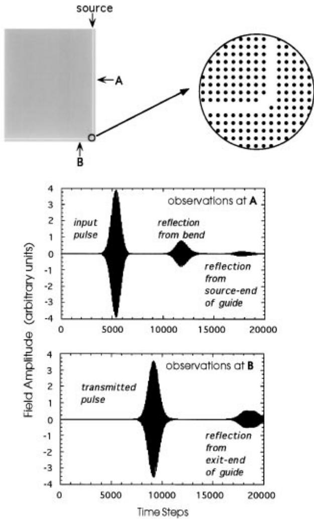
FIG. 1. Top panel: Schematic view of the  $100a \times 120a$  computational cell. The field amplitude is monitored at points *A* and *B*. The guide is located five lattice constants from the edge of the cell. Bottom panel: Field amplitude recorded at points *A* and *B*, as a function of time. The pulses reflected by and transmitted through the bend, as well as the pulses reflected from the edges of the cell, are easily discernible.
