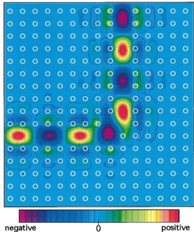
FIG. 2(color). Top two panels: Spectral profile of six input pulses. Computed transmission and reflection coefficients for each input pulse. The oscillations in transmission at low frequencies are numerical artifacts and are discussed in Ref. [9]. Bottom panel: Electric field pattern in the vicinity of the bend for frequency  $\omega = 0.353 \times 2\pi c/a$ . The electric field is polarized along the axis of the dielectric columns.
