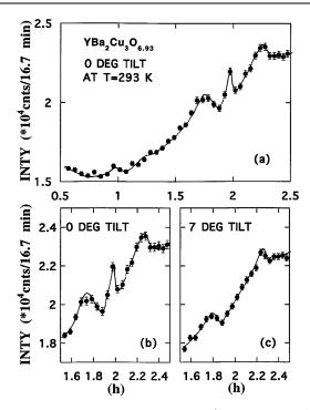
FIG. 2. (a) The result of a scan along  $\mathbf{b}^*$  or along the  $0^\circ$  line. (b) An expanded version of the scan while (c) is the result obtained along the  $7^\circ$  direction [see Fig. 1(b)]. Superlattice or satellite peaks are found around the Bragg peak positions for the larger Q reflections. Solid lines are guides to the eye.
