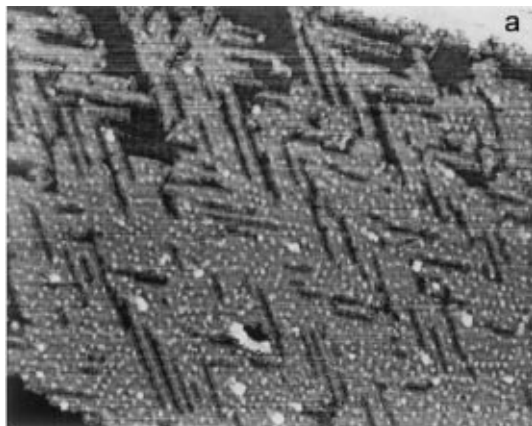
FIG. 4. Ni nanogratings on herringbone reconstructed Au(111) formed by nucleation at -0.62 V followed by a change to -0.64 V at the upper edge of the image ( I_t = 10 nA, 1420 \times 1130 \text{ \AA}^2 ).
