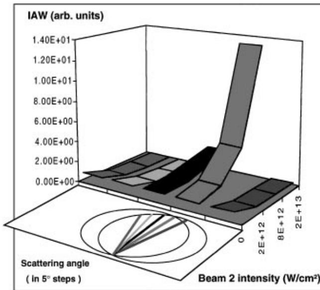
FIG. 4. Combined plot of the modified levels of ion acoustic waves from SBS for different directions, as a function of seed-beam intensity. Signals are normalized to 1 for  $I_{\text{seed}} = 0$ . The green line corresponds to the direction of resonance. The angular bandpass for each direction is  $5^\circ$ , in steps of  $5^\circ$ .
