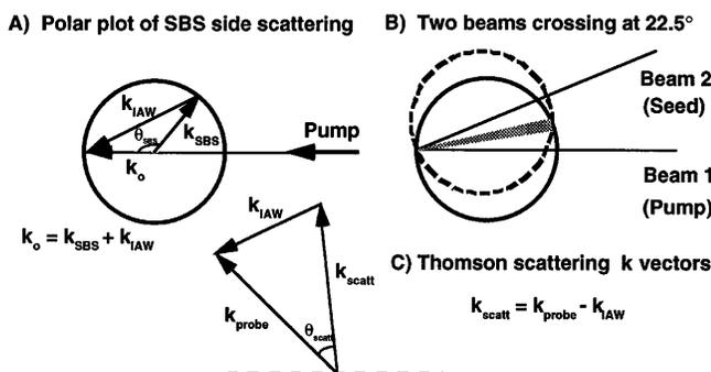
FIG. 1. Polar plot of ion acoustic waves of SBS for all scattering angles (a) and for the combination of two interaction beams separated by  $22.5^\circ$  (b), and Thomson scattered  $k$  vectors (c).
