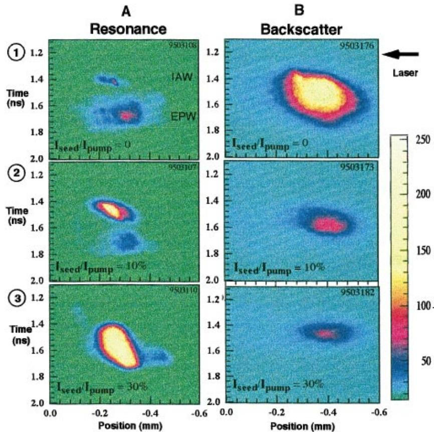
FIG. 2(color). Temporally resolved location of ion acoustic waves, along the direction of resonance (a), and along the direction of backscatter for the pump beam (b). The interaction beam arrives from the right, and the summit of the plasma is at position  $z = 0$ . The time scaled is referred to  $t = 0$  for the peak of the plasma forming beam. The seed beam to pump beam intensity ratio  $I_{seed}/I_{pump}$  is as follows for the different frames: (1) 0, (2) 10%, and (3) 30%.
