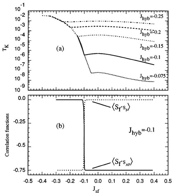
FIG. 2. (a) Kondo temperature as a function of  $J_{sf}$  for different values of  $J_{hyb}$  ( $B_F = B_{AF} = 1$ ) and (b) correlation function  $\langle \vec{S}_f \cdot \vec{S}_{AF} \rangle$  (solid line),  $\langle \vec{S}_f \cdot \vec{S}_f \rangle$  (dotted line), as a function of  $J_{sf}$  for  $J_{hyb} = -0.1$  from the Yosida method.
