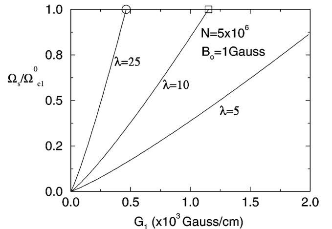
FIG. 1. The increasing spin-gauge effect for increasing field gradients and increasing oblateness of the trap. The square and circle indicate the appearance of vortex ground states, i.e., when  $\Omega_s / \Omega_{c1}^0 = 1$ .
