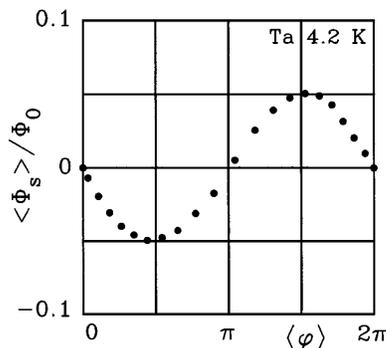
FIG. 4. The sinusoidal CPR of a tantalum point contact ( $T_c = 4.5$  K) measured at 4.2 K. The  $L^*$  of this tantalum MCBS is 0.16 nH.
