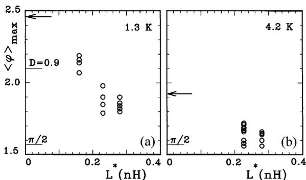
FIG. 3. In (a) and (b) the measured values of  $\langle \varphi \rangle_{\max}$  are plotted versus  $L^*$  for 1.3 and 4.2 K, respectively.  $L^*$  is the experimentally determined value  $L - M$  as it is defined in the text, and is 0.16, 0.23, 0.28 nH, respectively. Indicated are the predictions for a point contact with  $D = 1$  (arrows) and  $D = 0.9$ , without fluctuations.
