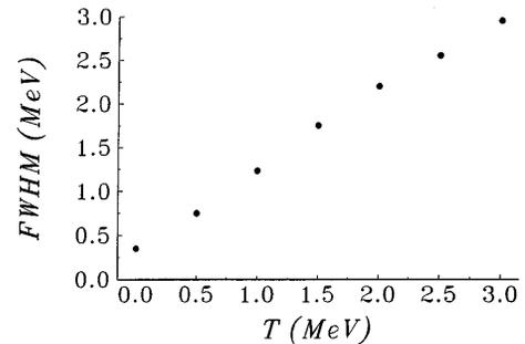
FIG. 3. Full width at half maximum of the strength functions of a single-particle state at the Fermi energy as a function of temperature.
