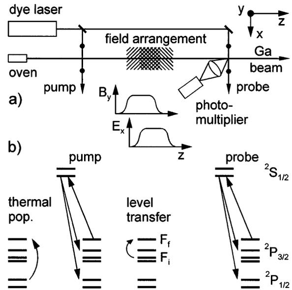
FIG. 2. (a) Sketch of the experimental arrangement; (b) scheme of the pump-probe detection. For details see text.
