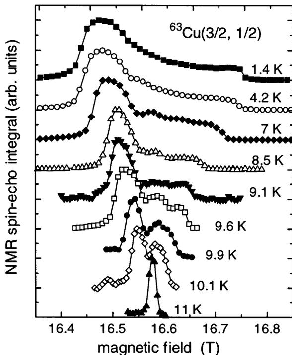
FIG. 4. Temperature dependence of the NMR line shape taken at 172.4 MHz.
