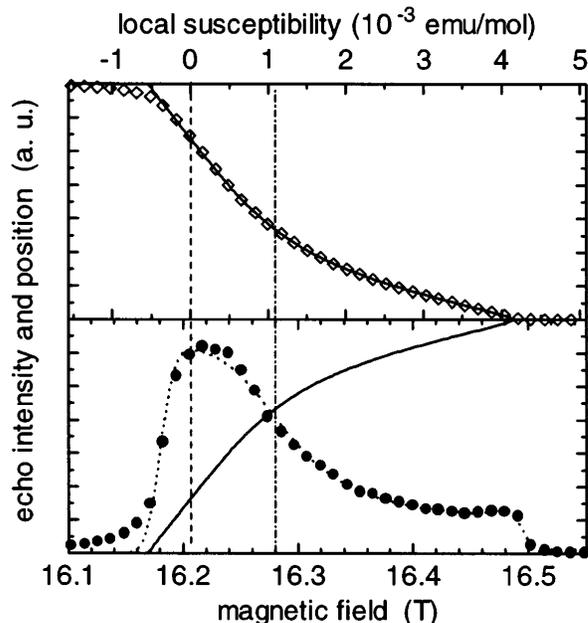
FIG. 2. The  $^{63}\text{Cu}$  ( $3/2 \leftrightarrow 1/2$ ) line shape (circles) taken at 1.4 K and 169.5 MHz, and the numerical integral of these data (diamonds). The lines are explained in the text.
