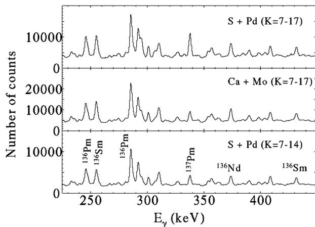
FIG. 3. Partial  $\gamma$ -ray spectra measured by the HPGe detectors for the S- and Ca-induced reactions. The selected BGO-multiplicity ( $K$ ) windows are indicated and strong  $\gamma$  rays emitted by the evaporation residues are labeled.
