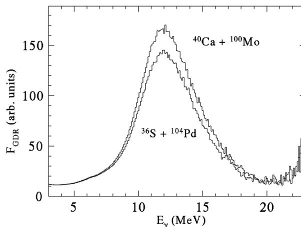
FIG. 2. Linearized plot of the experimental  $\gamma$ -ray spectra for the S- and Ca-induced reactions. The spectra were normalized in intensity between 3 and 4 MeV. The analysis was restricted to events having a BGO multiplicity  $K$  between 7 and 17.
