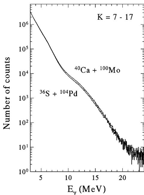
FIG. 1. Measured  $\gamma$ -ray spectra associated with the reactions  $^{36}\text{S} + ^{104}\text{Pd}$  and  $^{40}\text{Ca} + ^{100}\text{Mo}$  at bombarding energies of 160 and 170 MeV, respectively. The analysis was restricted to events having a BGO multiplicity  $K$  between 7 and 17. These spectra were normalized in intensity between 3.0 and 3.5 MeV.
