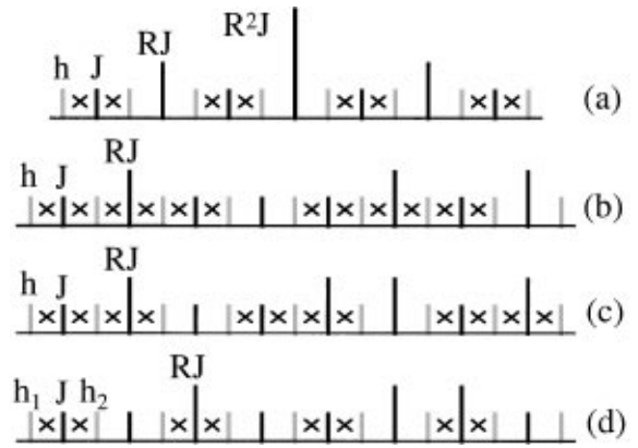
FIG. 1. Matrix-elements T_{j,j+1} as a function of j for different nonperiodic sequences: (a) hierarchical, (b) period doubling, (c) three folding, and (d) paper folding. Components of the eigenvector to be decimated out in the RG transformation are denoted by crosses. The heights of solid vertical bars indicate the strength of the couplings; the grey bars stand for the field.
