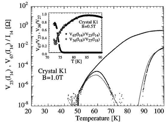
FIG. 4. Primary  $V_p(T)/I$  and secondary  $V_s(T)/I$  apparent resistances (points), and calculated secondary apparent resistance from the primary and  $c$ -axis voltages (solid line) for crystal K1 at 1.0 T. The inset shows the temperature dependence of the ratios  $V_{67}/V_{23}$  and  $V_{37}/V_{26}$  at 0.5 T for crystal K1.
