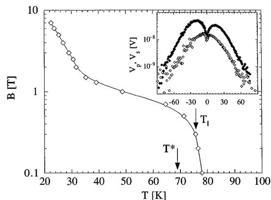
FIG. 2. The field dependence of the  $T_{\text{irr}}$ , where  $V_p$  vanishes for crystal K1. The line is a guide, and the temperatures  $T^*$  and  $T_l$  are discussed in the text. The inset shows  $V_p(\theta)$  and  $V_s(\theta)$  at 72.8 K and 0.5 T.  $\theta = 0$  corresponds to  $B//\text{defects}$ .
