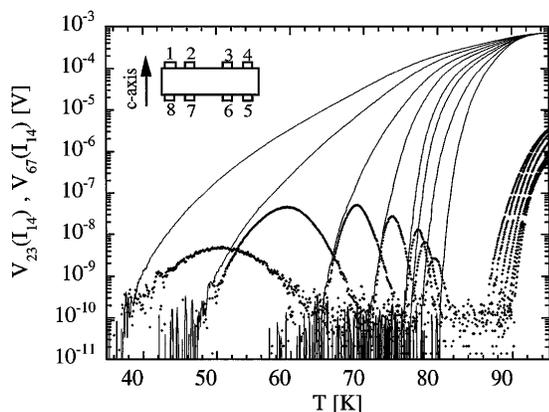
FIG. 1. Primary,  $V_{23}(I_{14})$  (solid line), and secondary,  $V_{67}(I_{14})$  (points), voltages for crystal K1 for  $B//c//\text{defects}$  of 0.1, 0.2, 0.3, 0.5, 0.7, 1.0, and 1.3 T.  $B_\Phi = 0.5\ \text{T}$ . The inset shows the contact configuration.
