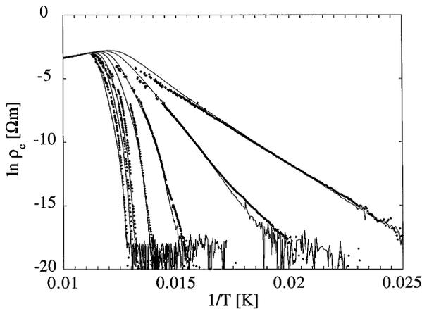
FIG. 3. Directly measured  $\rho_c$  extracted from  $V_{27}(I_{18})$  (solid lines) and from the FT data (points) as discussed in the text for the same fields as in Fig. 1.
