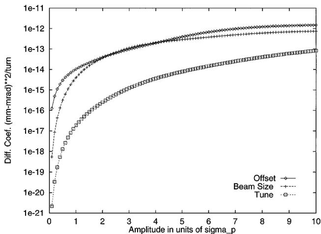
FIG. 3. Comparison of the diffusion coefficients in  $J$  due to tune fluctuations, offset fluctuations, and beam size fluctuations given by Eqs. (4), (8), and (9), respectively.  $\tau_c = 10.0$ ,  $\Delta\nu_r = 10^{-4}$ , and  $\Delta d_r = 0.01 = \Delta\sigma_r$ . Other parameters are the same as in Fig. 1.
