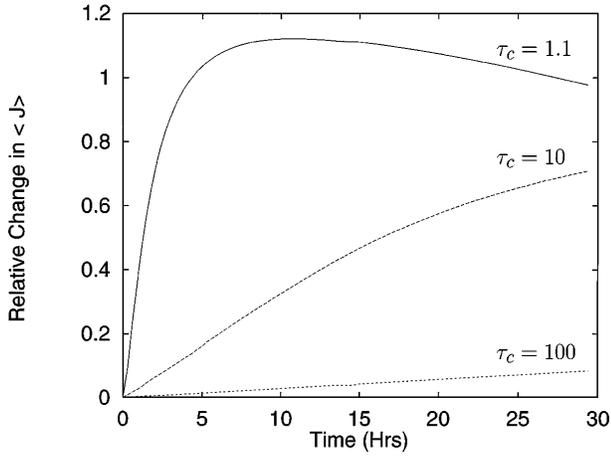
FIG. 2. Relative growth in the average action  $\langle J \rangle$  of a proton beam over a storage time of 30 h due to tune fluctuations at three noise correlation times. Parameters are the same as in Fig. 1.
