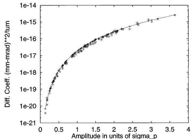
FIG. 1. The diffusion coefficient  $D_\nu(J)$  calculated analytically from Eq. (4) (dashed line) compared with the values obtained from the simulation.  $\sigma_p$  is the rms size of the proton beam. Parameter values  $\nu^0 = 0.291$ ,  $\Delta\nu_r = 10^{-4}$ ,  $\tau_c = 10$ ,  $N_{b,\text{op}} = 3.8 \times 10^{10}$ ,  $\gamma_p = 874$ ,  $\beta^* = 7.0$  m, and  $\sigma_{\text{op}} = 0.286$  mm.
