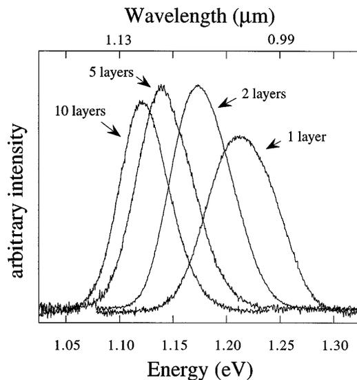
FIG. 3. 8 K photoluminescence of vertically stacked islanding layers showing the variation in spectral peak position and linewidth with the number of stacked islands.
