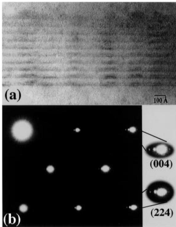
FIG. 1. (a) TEM image of several columns of vertically aligned InAs islands (dark regions). (b) Selected area diffraction pattern in TEM sample in (a) showing superlattice diffraction spots in the (001) growth direction.
