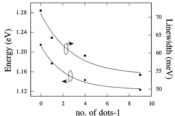
FIG. 4. Changes in spectral linewidth (a) and energy (b) are shown as a function of the number of vertical islanding layers. In each case, the exponential fit uses the same fitting parameter.
