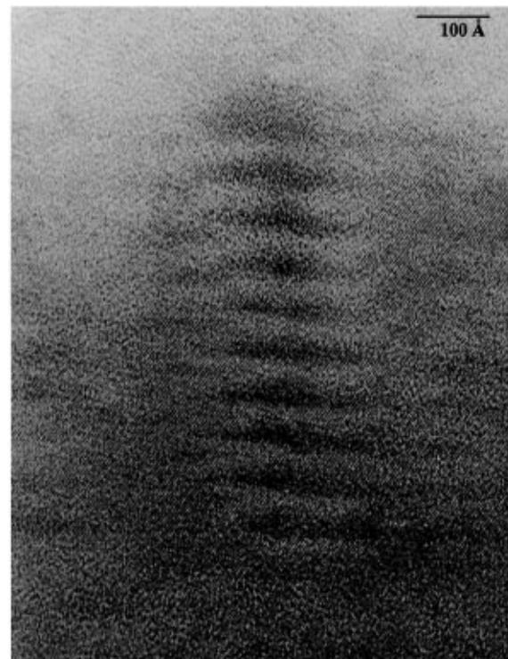
FIG. 2. TEM image showing one column of vertically aligned InAs islands. The island height is approximately  $40 \text{ \AA}$  and in the in-plane dimension is approximately  $180 \text{ \AA}$ .
