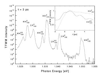
FIG. 3 Spectrally resolved four-wave mixing at  $\tau = 3$  ps showing the heavy hole and light hole biexcitons. Inset shows the four-wave mixing instensity of the heavy hole exciton and biexciton as a function of delay.
