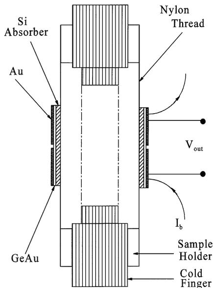
FIG. 1. Schematic cross section of a detector mounting, viewed from the  $90^\circ$  source position. The planes of the detectors are perpendicular to the page, with the thermistor sides facing outward. The sample holder has a hole giving a clear path in vacuum from one detector to the other.
