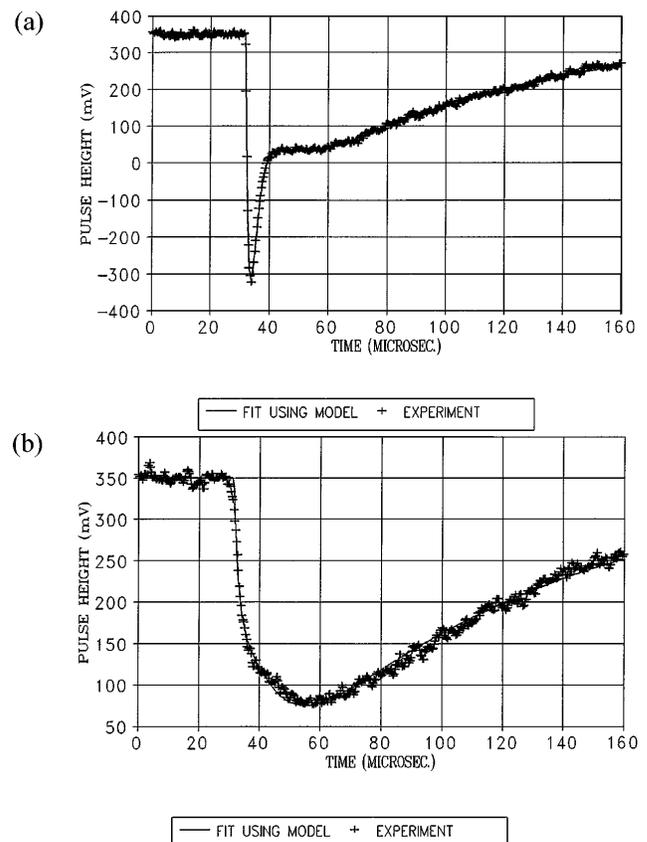
FIG. 2. (a) Characteristic pulse from particle penetrating GeAu thermistor and depositing energy directly in the thermistor itself. (b) Characteristic pulse from nonpenetrating particle.
