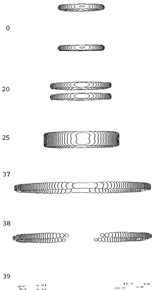
FIG. 1. Symmetric annihilation of two vortex rings; (dimensionless) times shown are 0, 20, 25, 37, 38, and 39.
