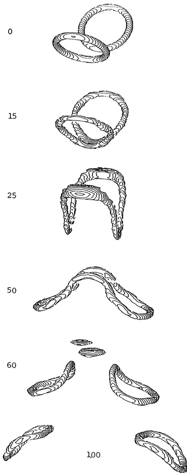
FIG. 2. In-plane collision of two vortex rings at  $90^\circ$  incidence, seen from the side. Times 0, 15, 25, 50, 60, and 100.
