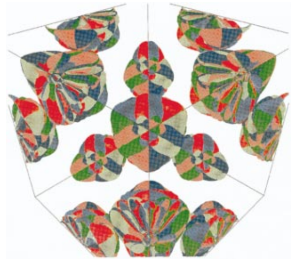
FIG. 3 (color). Isosurfaces of the components of the magnetization density along [1\bar{1}0] (blue), [\bar{1}01] (red), and [01\bar{1}] (green), calculated for the case of the average moment along the [111] direction are shown for the same cube as in Fig. 1 but viewed from the [111] direction. Both positive (darker colors) and negative (lighter colors) values are plotted, and the same isovalue is used as in Fig. 1.
