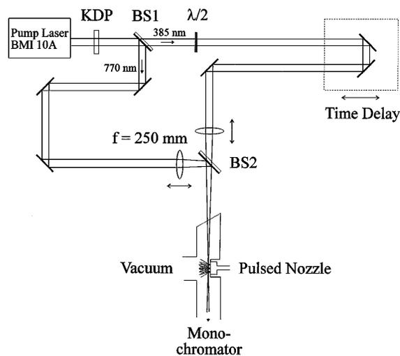
FIG. 1. Experimental setup. Beam splitters (BS) are highly reflective for 770 nm.
