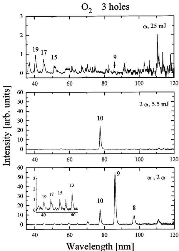
FIG. 5. Comparison of high-order harmonic spectra generated in three  $O_2$  gas jets (three open holes) at a backing pressure of 330 mbar.
