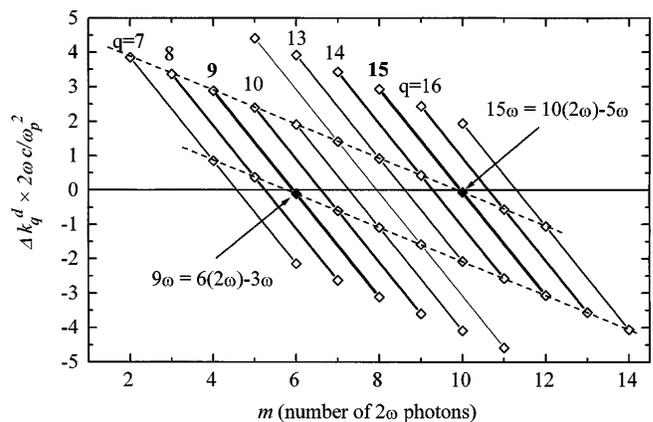
FIG. 2. Dispersive phase mismatch for two-color mixing process  $\omega_q = m(2\omega) - l\omega$ , where  $q = 2m - l$ . The harmonic order is constant along the solid lines. The transition from one point to another along the dashed lines corresponds to the transformation  $q \rightarrow q + 1$ ,  $m \rightarrow m + 1$ , and  $l \rightarrow l + 1$ .
