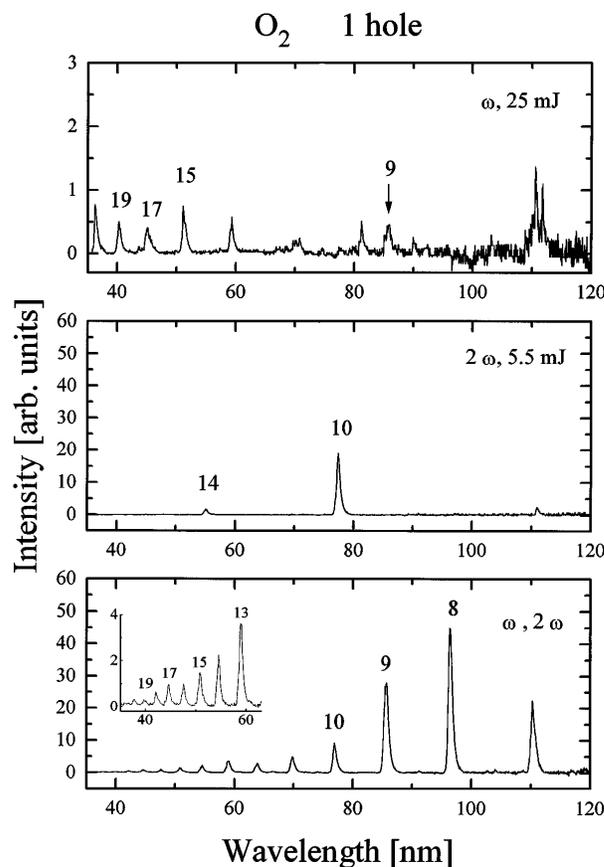
FIG. 4. Comparison of high-order harmonic spectra generated in a single  $\text{O}_2$  gas jet at a backing pressure of 330 mbar by fundamental radiation ( $\omega$ ), by second harmonic ( $2\omega$ ), and by two-color ( $\omega, 2\omega$ ) laser radiation. The spectral sensitivity of the detection system has been taken into account.
