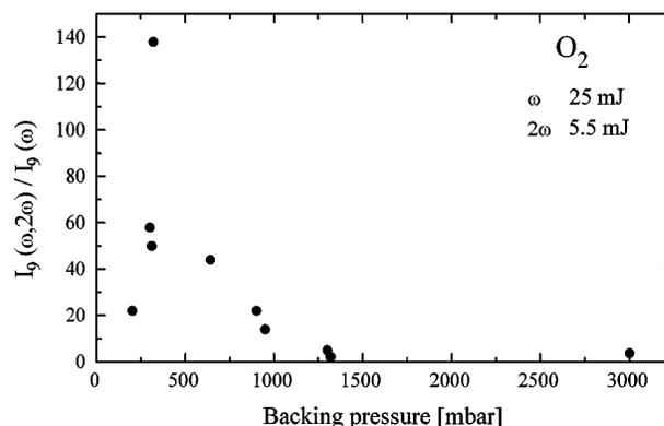
FIG. 3. Ratio of the 9-order harmonic signals generated in a single  $\text{O}_2$  gas jet by two-color ( $\omega, 2\omega$ ) laser radiation and by the fundamental radiation alone. Approximately 100 shots are used for each experimental point.
