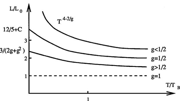
FIG. 1. Lorentz number  $L$  for transport through a single impurity versus temperature, for several values of  $g$ .
