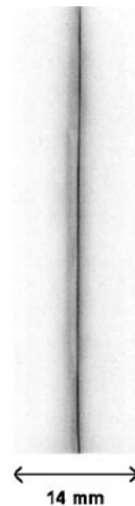
FIG. 2. Shock generated plasma column on axis (inner diam \leq 500 \mu\text{m} , length = 90 mm) for a discharge current of 40 kA, at an exposure time of 5 ns.
