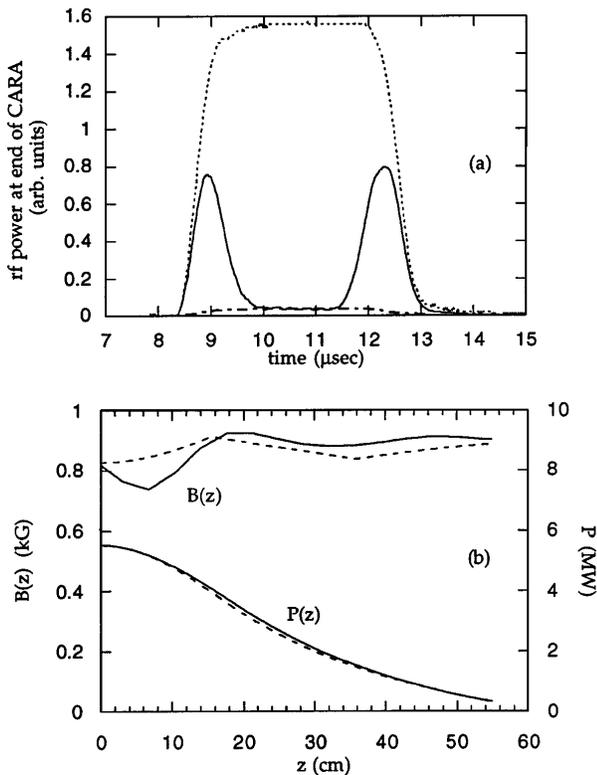
FIG. 2. (a) Pulse shape of rf power at the end of CARA with (solid line) and without (dashed line) the injected beam. The lower dashed trace is the same as the upper, but attenuated by 12 db. (b) Idealized (dashed line) and actual (solid line) profiles of magnetic field  $B(z)$  along CARA, and rf power profiles  $P(z)$  calculated for each.
