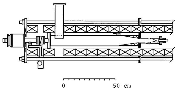
FIG. 1. Schematic of CARA used in experiments reported in this Letter. Shown (from left) are the electron gun, pumping port, gate valve, waveguide input (one of two), CARA waveguide (internal tapers not shown), rf sample point, conical absorber, beam collector, individually powered field coils, and flux bars.
