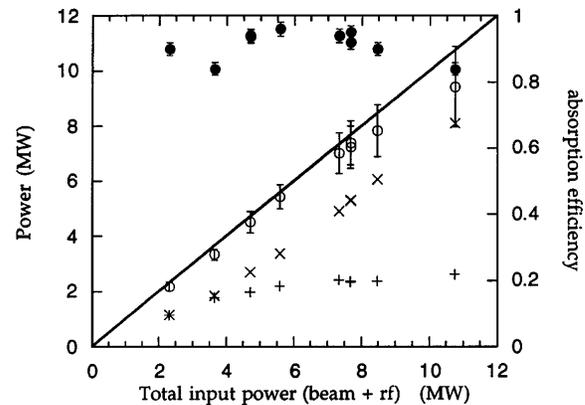
FIG. 3. Total beam power (O), efficiency (●), CARA injected beam power (+), and initial rf power (x) plotted versus total input power. The solid line corresponds to 100% efficiency.
