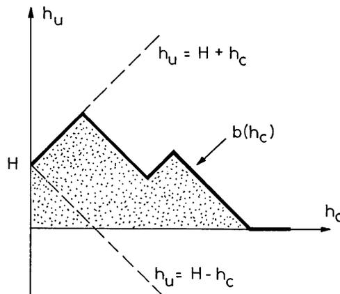
FIG. 1. Preisach representation in the  $(h_c, h_u)$  plane, showing the region of integration (point filled) for Eq. (2) and lines controlling  $b(h_c)$  behavior according to  $H - h_c \leq b(h_c) \leq H + h_c$ .
