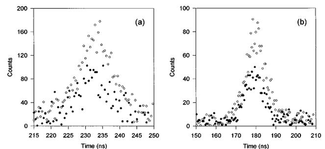
FIG. 2. Positronium time-of-flight spectra taken at (a) 39.6 eV and (b) 63.5 eV incident positron energies. The hollow circles refer to the Ps beam incident onto an Ar target. The filled symbols represent the Ps beam intensity transmitted through the target. Target pressures are given in the text.
