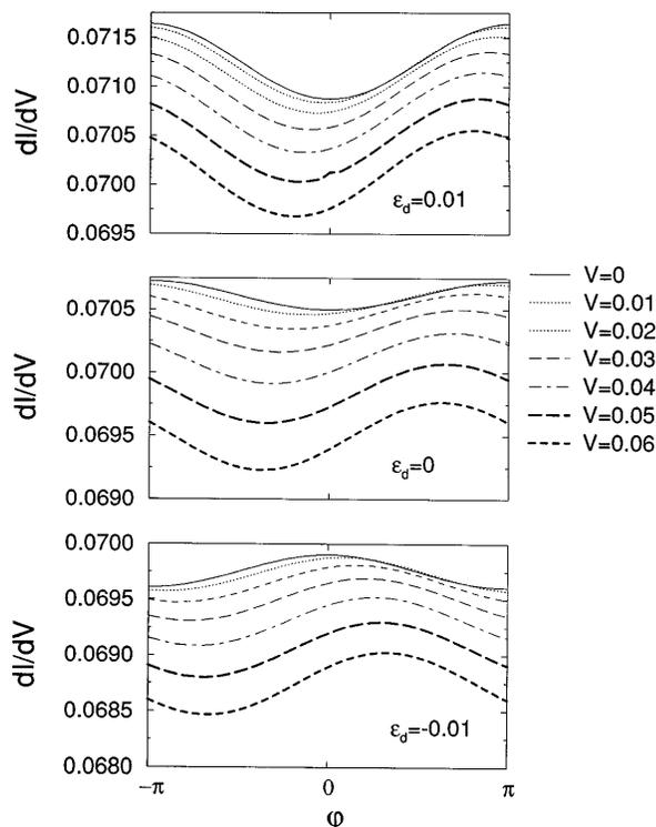
FIG. 3. Differential conductance (in units of  $e^2/h$ ) for the case of weak transmission ( $t = 0.1$ ) as a function of magnetic flux for various voltages and positions of the level in the dot ( $T = 10\Gamma = 0.1$ ,  $M = 2$ ). Note that the linear conductance ( $V = 0$ ) is symmetric around  $\varphi = 0$ , whereas there is no such symmetry in the nonlinear response case.
