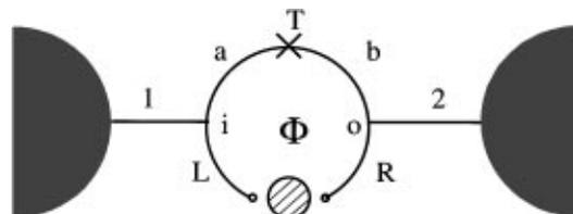
FIG. 1. Geometry of the model system studied here. Leads 1 and 2 connect to the left and right reservoirs (shaded). The ring is connected to a quantum dot via high tunneling barriers.  $\Phi$  is the flux penetrating the ring.
